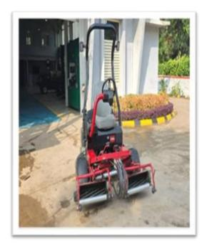
Our existing hydraulic triplex mower, purchased in 2017, has accumulated 4,800 running hours and is now nine years old, approaching its expected lifespan of 6,000 hours. In 2022- 2023, the mower spilled hydraulic oil onto the greens three times (green 13, green 16, and the 11th approach), and in 2023-2024, there were four additional oil spill incidents (green 11, green 6, green 18, and green 8).
